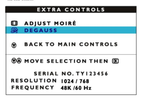
5) To degauss your screen, press the button. Your screen will be degaussed, then the MAIN CONTROLS window will reappear. CLOSE MAIN CONTROLS will be highlighted.
